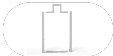
Door Frame with Monorail Channel
